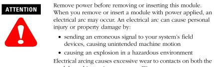
Electrical arcing causes excessive wear to contacts on both the module and its mating connector. Worn contacts may create electrical resistance.
